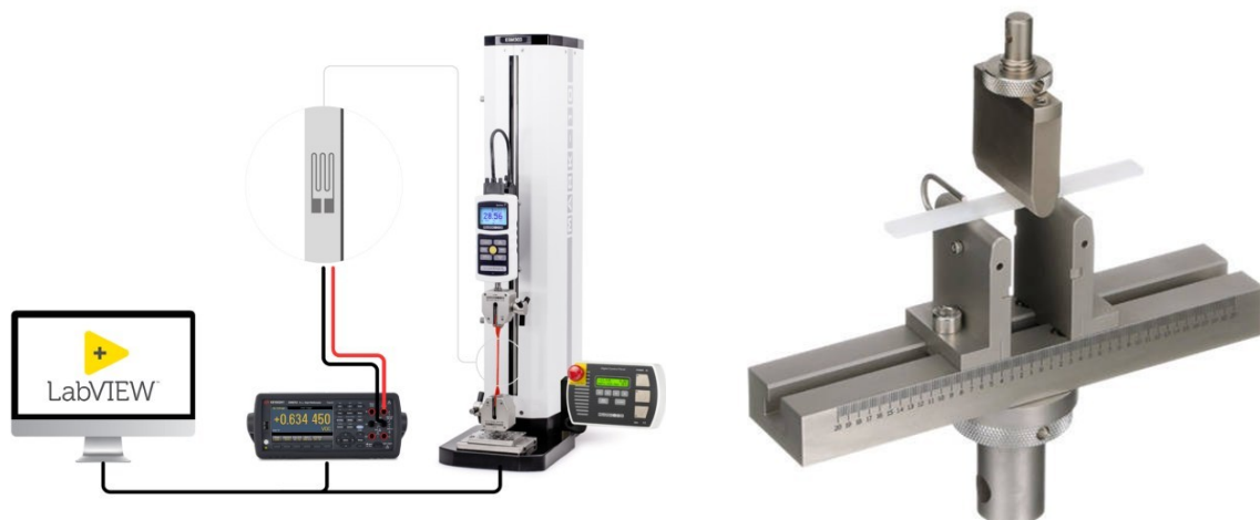
Figure 3. Electromechanical validation setup and three-point bending fixture used for titanium specimens.
